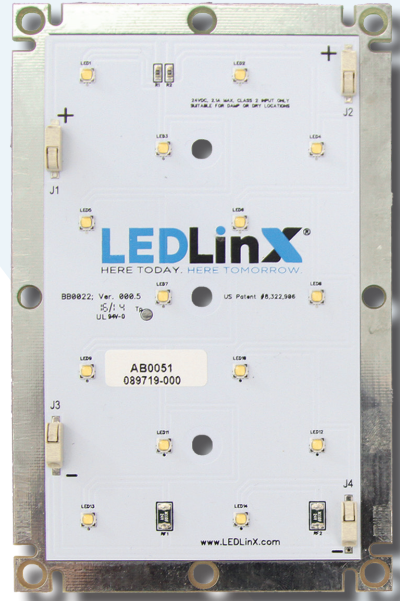
High Power Rectangle AB0051 - Luxeon Type T 7W - 28W per module
